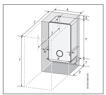
Fig. 9 Appliance minimum clearances
