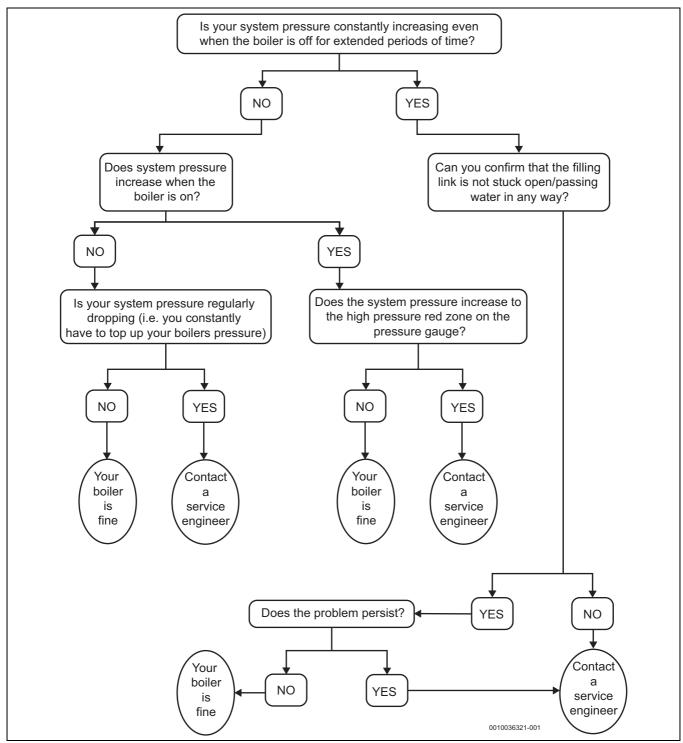
Fig. 10 Gassing flow chart
